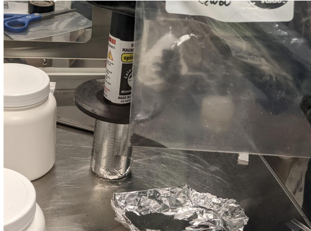
Fig. 24. Checking magnetic response of the simulant samples.
