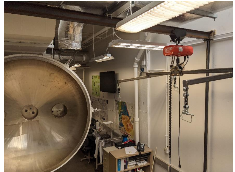
Fig. 29. More equipment/hardware on chamber facility upgrade (LN2 shroud and tanks, and crane).
