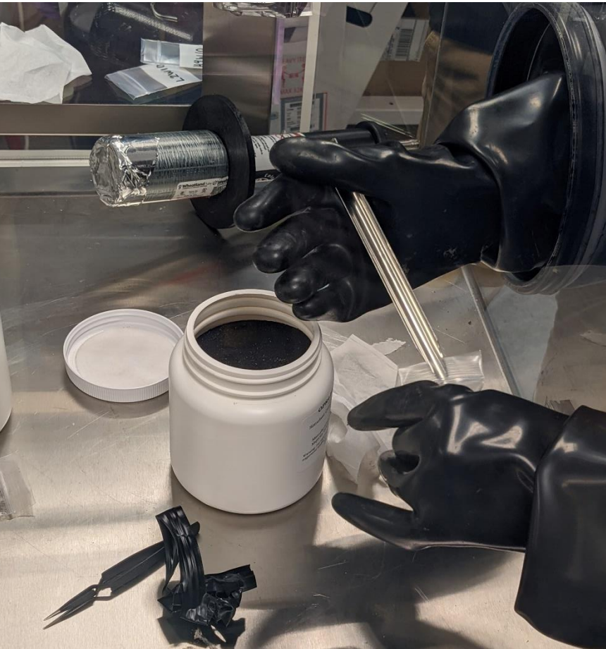
Fig. 24. Checking magnetic response of the simulant samples.
